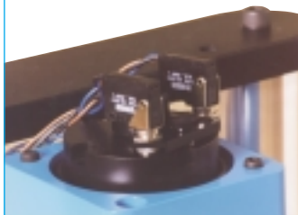
Close up of limit switches for monitoring brake pad wear state and actuator position (On or Off)
